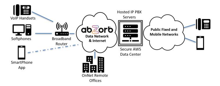
As per the diagram, the main difference between hosted voice and traditional voice solutions is that all your telephones (handsets or softphones) are connected directly to your I router via your data local area ethernet network. All the intelligent functionality (call recording, call routing, hunt groups, time of day settings etc.) is done in the secure cloud instead of using onsite expensive telephony hardware.
